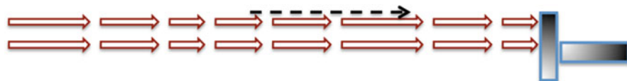
Fig. 7.3 The arrows now represent oscillations along the same direction as the wave travel, a longitudinal wave; in this case they will all go through regardless of the orientation of the slits
