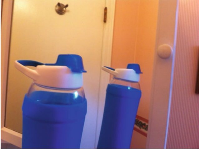
Fig. 3.7 The reflection of the plastic bottle exhibits a well-known but often misunderstood property of plane mirrors. The orientation is unchanged since the handle appears on the left side of both the object and its image; what changes is the front-to-back perspective. The back of the object appears as the front of the image
