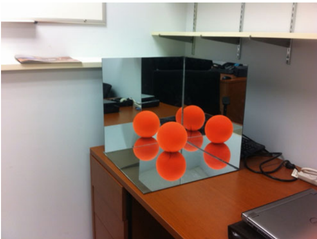
Fig. 3.8 Placing three plane mirrors at right angles to each other will produce a number of reflections of the single object placed in front of them
